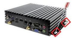
4. Then tighten up the other two screws in the marked positions on the other rack.
