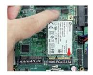
Insert the gold-figure side of the compatible MSATA card into the slot at a 30 degree angle and press down.
