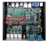
Locate the SO-DIMM slot on the board.
