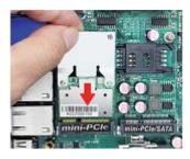
Insert the gold-figure side of the compatible WI-FI card into the slot at a 30 degree angle and press down.
