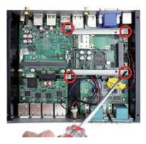
Remove the screws in the marked positions with a screwdriver to remove the HDD racks from the board.
