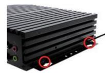
Install wall mount rack to the system by tightening two screws in the marked positions.
