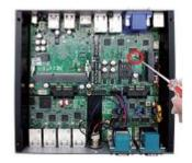
2. Remove the marked screw and use it to lock WIFI card to the slot in later installation.
