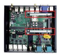
1. Locate HDD racks on the board. 2.
