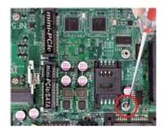
2. Remove the marked screw and use it to lock MSATA card to the slot in later installation.
