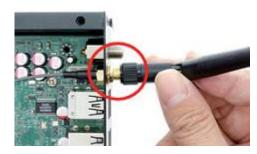
Connect the external Wi-Fi receiver antenna to the antenna connector on the rear panel.
