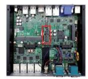
Locate the full-size MSATA / Mini-PCIE slot on the board.
