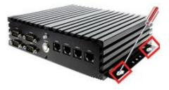
Wall mount the system by tightening two screws in the marked positions.
